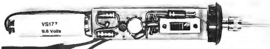
Photo shows component mounting details and location of battery bracket/connector at left end of pc board.
